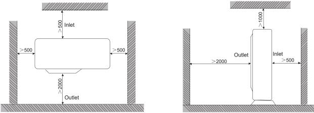
Note: In conderation of space restriction, for the left-handed figure, except the outlet side, distance between the unit and the nearest barrier at other three sides are allowed to be no less than 300mm; for the right-handed figure, distance between the inlet side and the nearest barrier is allowed to be no less than 300mm.
