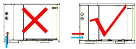
It is recommended to connect water pipe in horizontal direction. Do Not connect water pipe in vertical direction.
