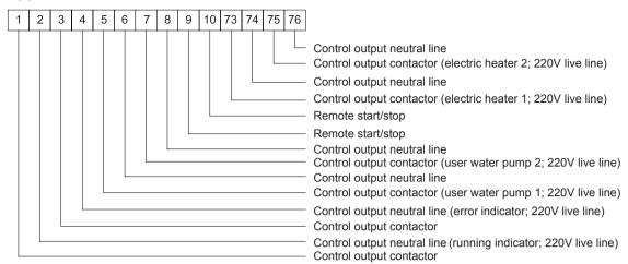
Note: the output control lines of the AC contactors for the auxiliary electric heater 1, auxiliary electric heater 2 can be wired to the corresponding wiring board of all units, while those for the error indicator and external passive contact switch should be wired to the corresponding wiring board of all units.
