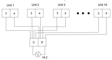
When it is required to display errors of several units, the wiring terminals (3,4) of each unit should be wired to the wiring terminals HL2 (C,D) of the error indicator. (If it is required to display the error of each unit independently, then the error indicator of each unit should be wired independently to the corresponding error output wiring terminals (3,4) of each unit.
