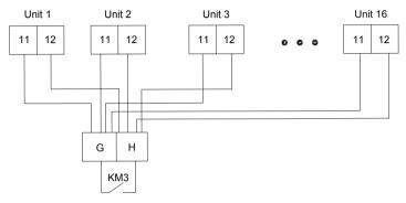
When one auxiliary electric heater serves more than one modules, its wiring terminals 11 and 12 are connected to terminals G and H respectively of an AC contactor marked with KM3.
