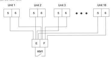
When multiple modules have direct control over one water pump, wiring terminals 5 and 6 for one modular unit are connected to terminals E and F respectively of the AC contactor (KM1) for the water pump, or 7 and 8 to E and F respectively of an AC contactor (KM2).
