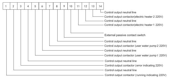
Note: the output control lines of the AC contactors for the running indicator, water pump 1, water pump 2, auxiliary electric heater 1, auxiliary electric heater 2 can be wired to the corresponding wiring board of all units, while those for the error indicator and external passive contact switch should be wired to the corresponding wiring board of all units as shown in the figure below.
