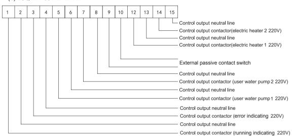
Note: the output control lines of the AC contactors for the auxiliary electric heater 1, auxiliary electric heater 2 can be wired to the corresponding wiring board of all units, while those for the error indicator and external passive contact switch should be wired to the corresponding wiring board of all units.
