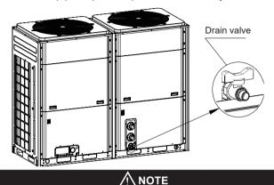
Keep the purge value of the water system open in order to drain the evaporator and condenser completely.
