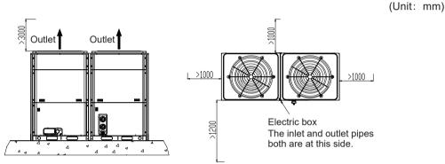
Note: The unit should be installed where at least 3 sides of the unit are not blocked.
