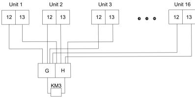
When one auxiliary electric heater serves more than one modules, its wiring terminals 12 and 13 are connected to terminals G and H respectively of an AC contactor marked with KM3
