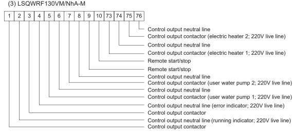
Note: the output control lines of the AC contactors for the auxiliary electric heater 1, auxiliary electric heater 2 can be wired to the corresponding wiring board of all units, while those for the error indicator and external passive contact switch should be wired to the corresponding wiring board of all units.
