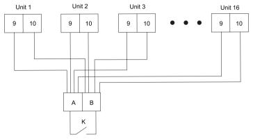
When external passive contact switch is available for multiple units, the wiring board 9 and 10 of each unit should be wired to the dry contact A and B.
