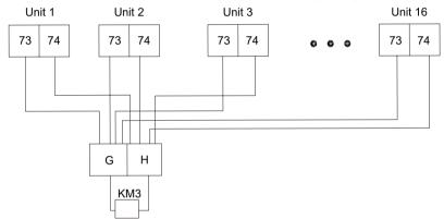
When one auxiliary electric heater serves more than one modules, its wiring terminals 73 and 74 are connected to terminals G and H respectively of an AC contactor marked with KM3
