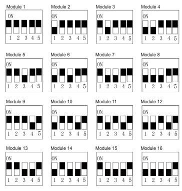
Note: the black block represents where the projecting lever of the DIP switch is.
